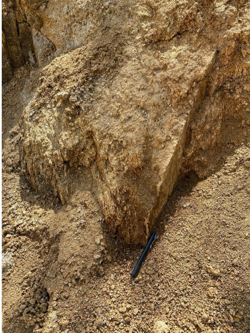
Figure 9: Shear Plane (parallel to pencil) and closely-spaced Joints in the Mackay granite. Joints are oriented N29W 90 and the shear plane is oriented N26E 90, defining a \sim 55^\circ angle of intersection. Approximate location is 1723830E/810820N.
