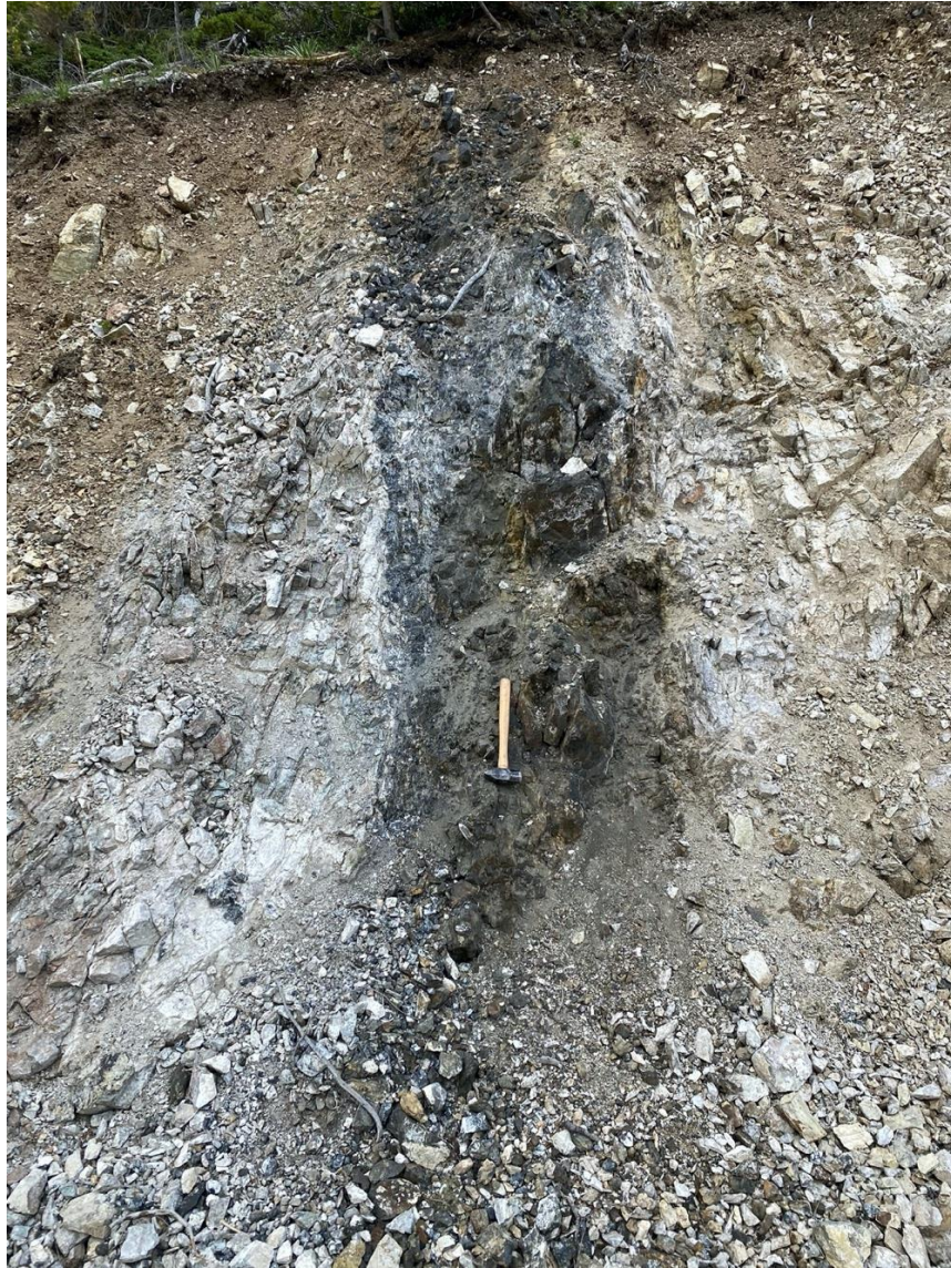
Figure 6: Massive magnetite vein about 3' wide cutting through endoskarn hosted by Granite Porphyry, with contacts oriented N9E 80NW. Approximate location is 1724747E/ 811110N.
