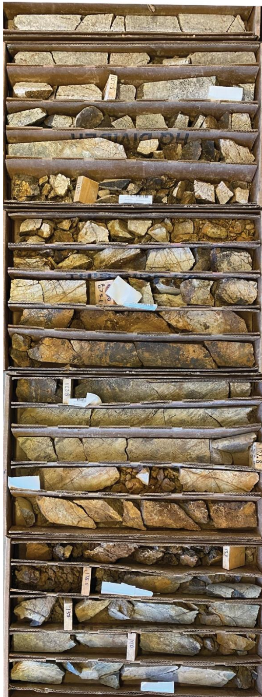
Figure 1: Core recovered from depths of 104'-143' in drillhole RSD20-02, located beneath the Red Star adit.
