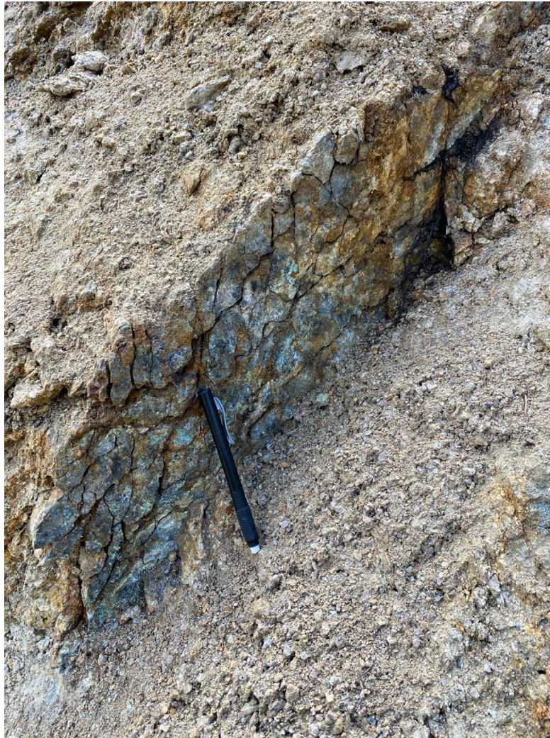
Figure 7: Shear Plane cutting through Mackay Granite with copper oxide minerals precipitated on the surface. Shear plane orientation is N39E 87SE. Approximate location is 1723760E/810850N
